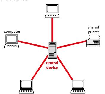
In a star network each device has a single connection to a central computer device.
