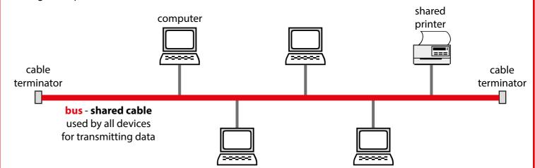
All devices are connected together through a shared communication cable, called a bus.
