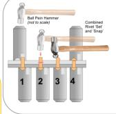
Rivets (aka Rivits) have various designs of head at one end and are used to fasten materials together by being passed through a punched or drilled hole and hammered over (usually) to form a head on the reverse side. They are available in several materials and sizes. can be solid or hollow and specialised designs also exist (e.g. 'Pop' Rivets).
