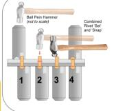
Rivets (aka Rivits) have various designs of head at one end and are used to fasten materials together by being passed through a punched or drilled hole and hammered over (usually) to form a head on the reverse side. They are available in several materials and sizes, can be solid or hollow and specialised designs also exist (e.g. 'Pop' Rivets).
